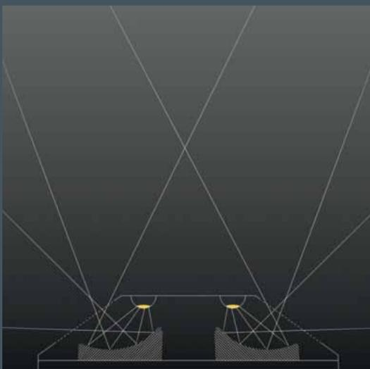
With the precise optical system the intensity of the light beam is adapted to varying distances from the luminaire to the window frame. Hence an optimal uniformity is achieved. Arclux RGBW creates the same effect with excellent colour mixing.
